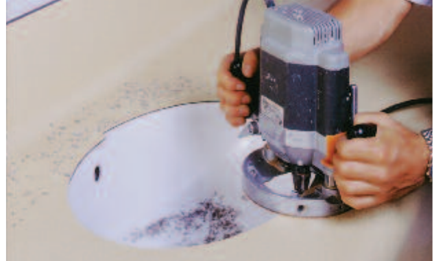
4. Mill the projection of the Compact Laminates flush on the visible side with a manual surface miller (angled miller!).
